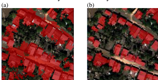
Figure 1 (a) Separating building from trees and (b) separating buildings based on elevation.
