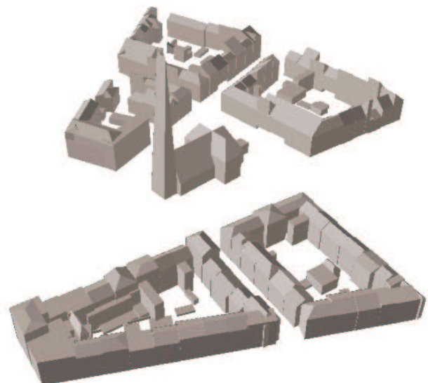
Figure 6: City model from Karlsruhe. Reconstructed using LIDAR data.
