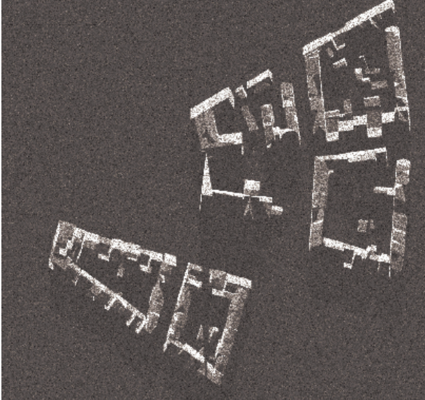
Figure 7: Simulated SAR image based on given 3D city model
