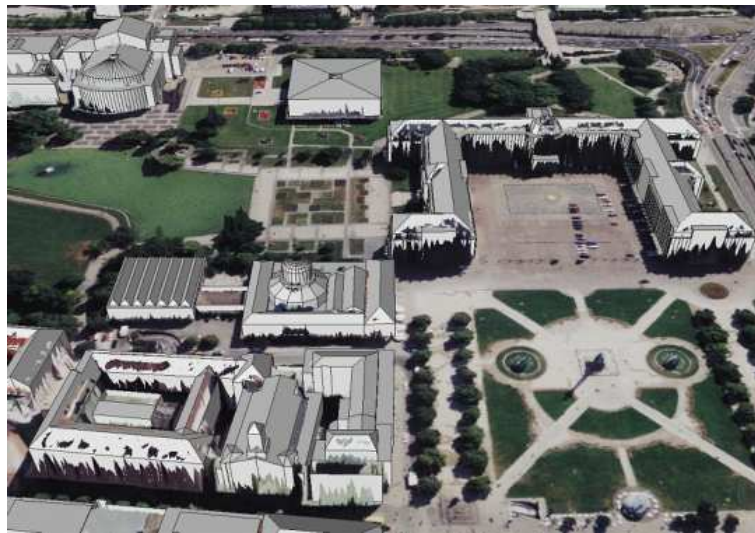
Figure 5: Extracted CAD-models overlaid to LIDAR DSM
