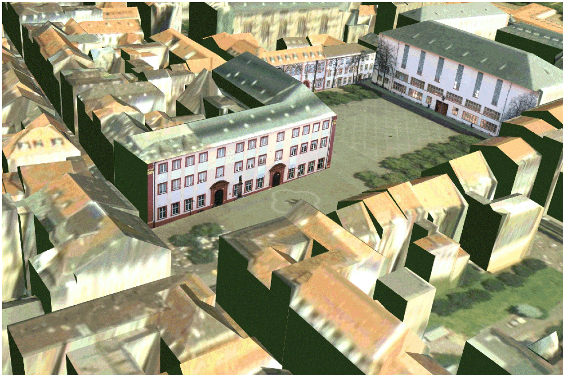
Figure 9: Visualization based on combination of aerial images and terrestrial texture
