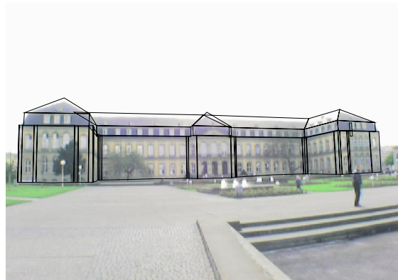
Figure 11: Projection of building based on refined orientation.
