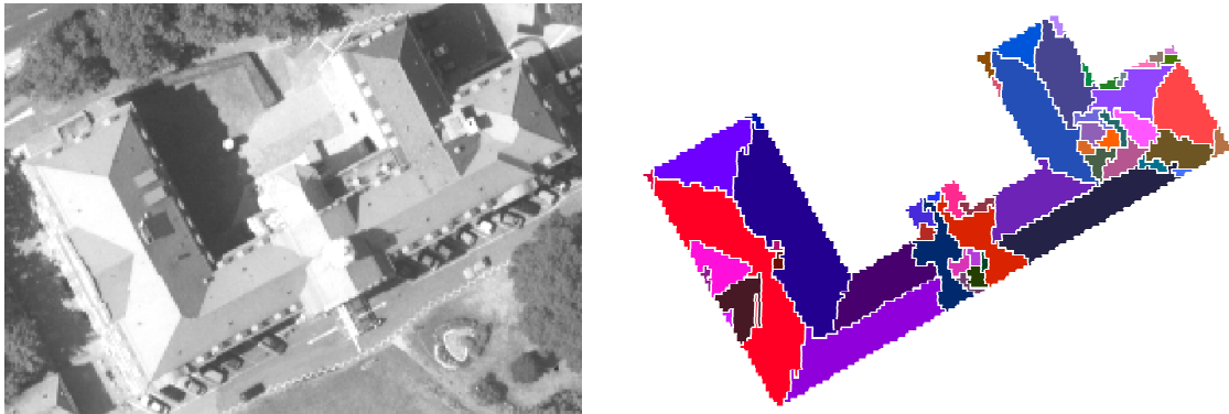
Figure 5. Left: aerial image of a building with complex roof. Right: regions obtained from a planar DSM segmentation.
