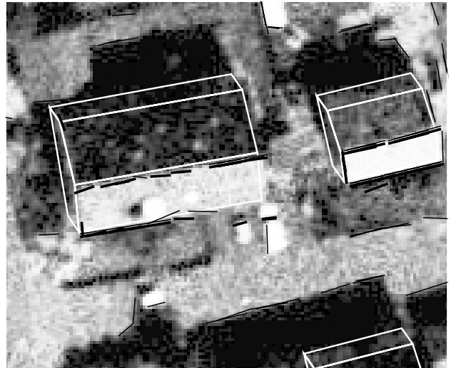
Figure 5: Constructed 3D building hypotheses projected to image (white) and matched image lines (black)
