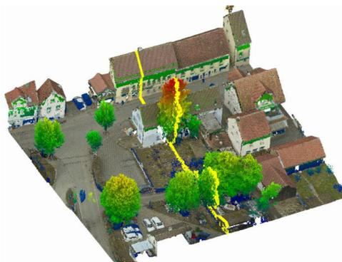
**Figure 7:** Comparison of 3D points from MVS (RGB) and LiDAR measurement (height coded). Yellow line defines profile depicted in Figure ??.
