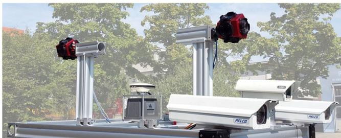
**Figure 10:** Multi-view multi-sensor configuration of the mobile mapping system of the Institute of Geomatics (IGEO), University of Applied Sciences and Arts Northwestern Switzerland (FHNW), which was used for capturing a dataset in Basel in August 2015.
