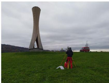
**Figure 5:** Network measurement when measuring the fixed point network.
