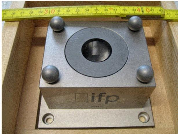
*Figure 20: Image of the calibration body for the multi sensor calibration; the four spheres yield the triangulation sensor's position; the cylindrical bore hole with its additional features in the inner part of the body yield the interferometers position.*
