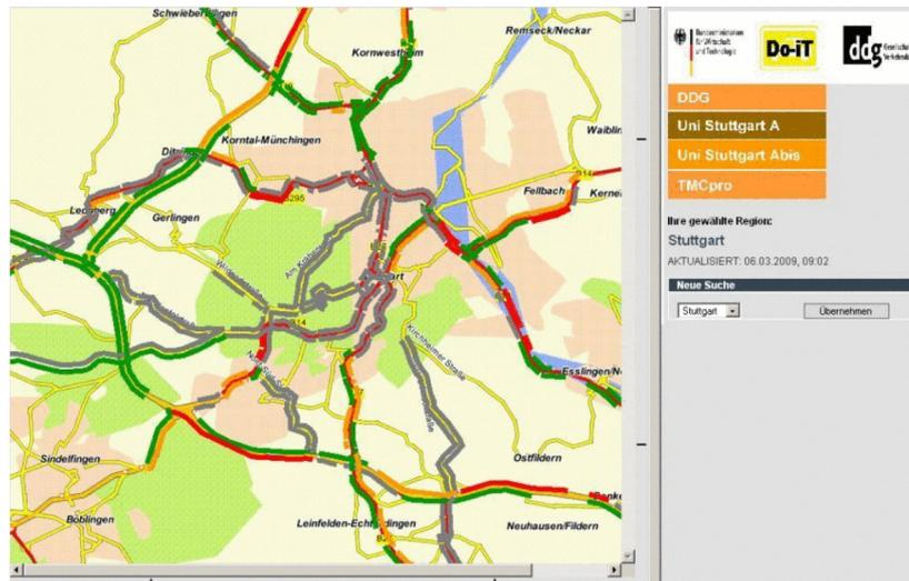
Figure 3: Forecast of traffic state with A-data
