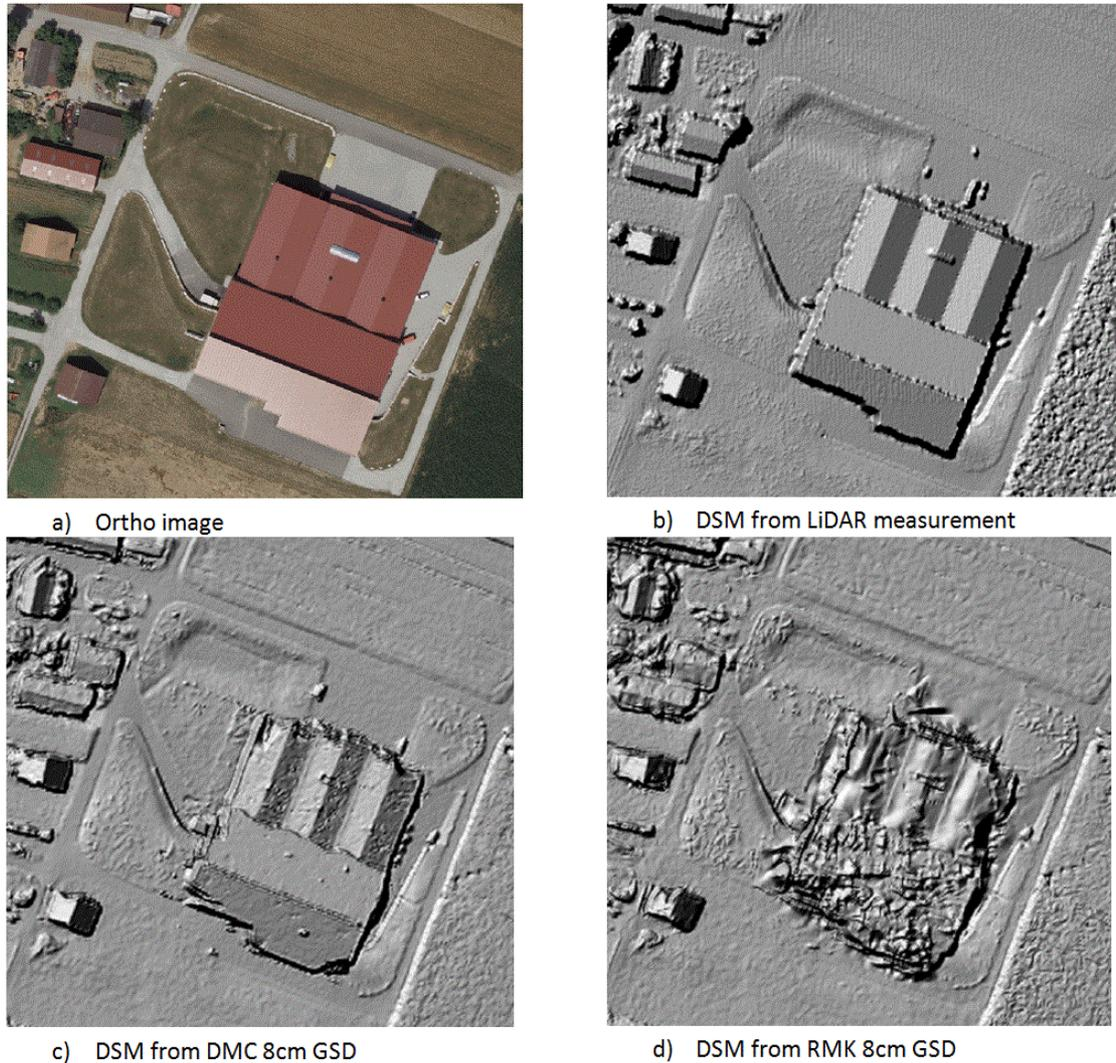
Figure 12: Comparison of shaded DSM from different data sets.
