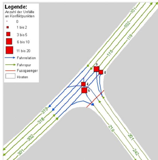
Fig. 12: Distribution of accidents at points with crossing manoeuvres
