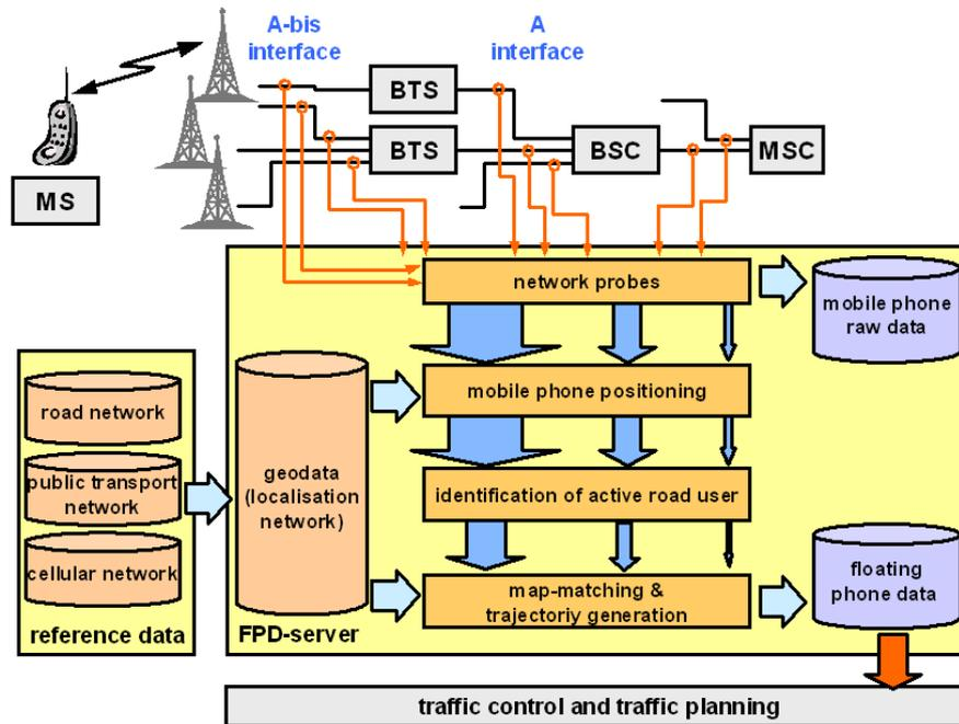
Fig. 13: System architecture and information flow for generation of Floating Phone Data within the project Do-iT
