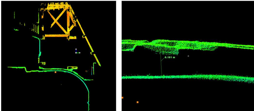
*Figure 15: Vertical section through the data, combining scan data from inside the church and from inside the truss. The thickness of the dome ceiling can be directly measured from the data.*
