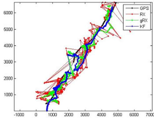
Fig. 3: Estimated trajectory: RX-Matching, smoothing (gRX), Kalman filter (KF)
