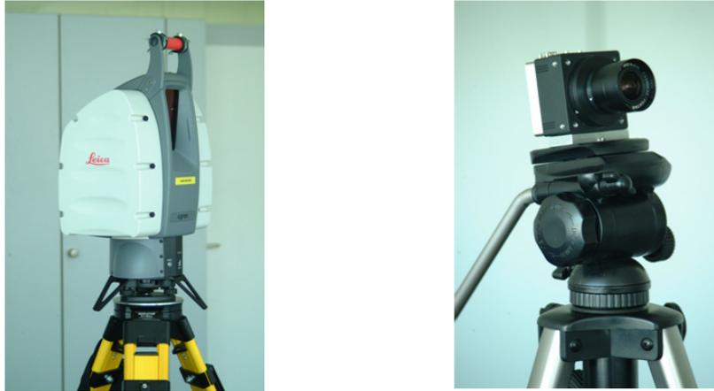
*Figure 16: The sensors utilized for this study are a laser scanner and a machine vision camera. The laser scanner to the left is a Leica HDS 3000. The camera to the right is a Basler A302f. Both devices were mounted on a tripod during data acquisition. The camera was moved using a dolly.*
