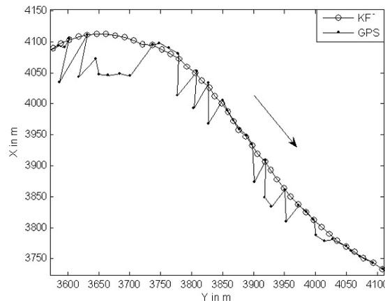
Fig. 1: Improved filtering through correct stochastic models (KF = Kalman filter)
