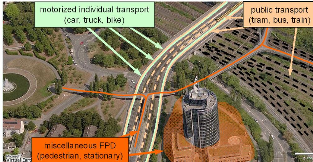
*Fig. 8: Identification of mobile subscribers for acquisition of individual traffic states*
