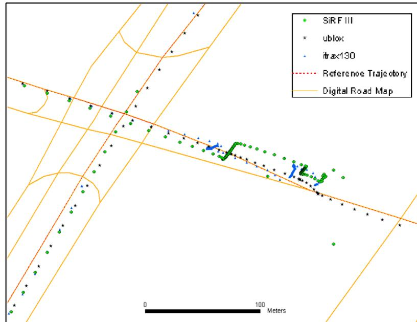
Fig. 7: Comparison of the positions provided by several low-cost GPS sensors in case of an underpass (North-South trajectory) and a tunnel (East-West trajectory)
