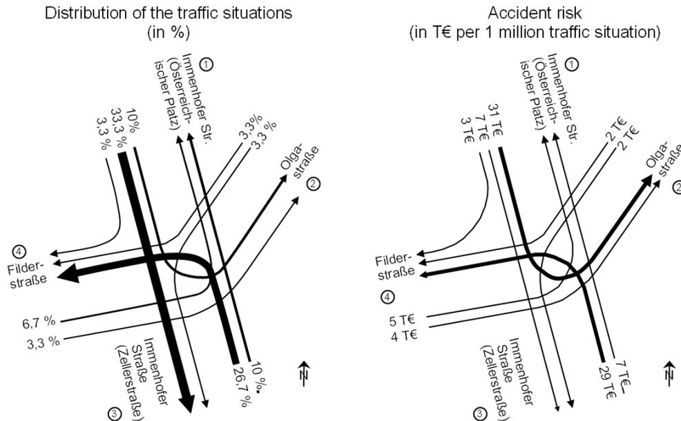
Fig. 10: Accident diagramm of distribution of accidents and accident risk for intersection Immenhofer Str. / Olgastr. / Filderstr. in Stuttgart
