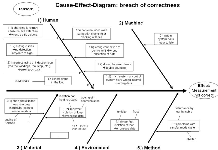
Fig. 9: Example - CED for examination of an induction loop for correctness
