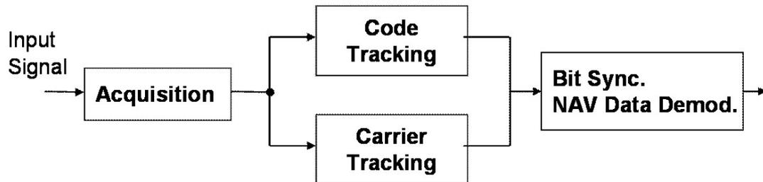
*Fig. 3: Flow diagram of the signal processing.*
