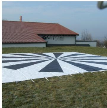
*Figure 9: Siemens star for geometric resolution determination.*
