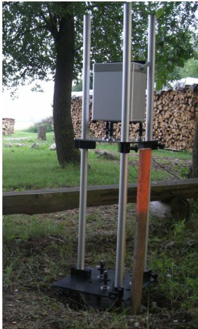
*Figure 13: Tripod of BKG with CG-5 in the upper level*
