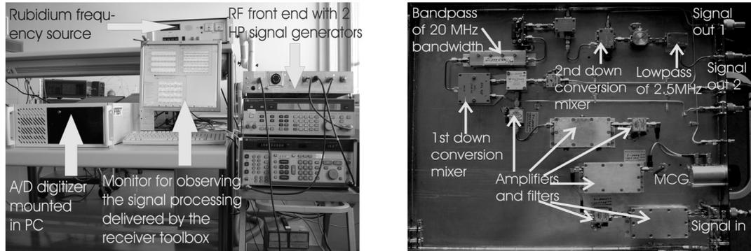
Fig. 1: Labor system for data collection: complete system (left); RF front end (right)
