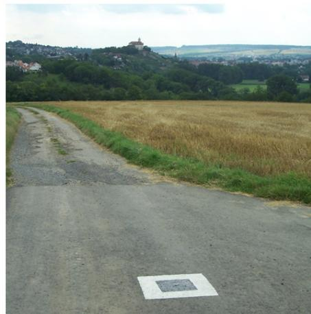
Figure 7: Signalized ground control point Vaihingen/Enz.
