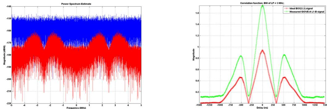
Fig. 2: Power spectral density (left) and autocorrelation function (right) of the GIOVE-A L1 open service signal
