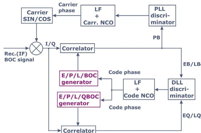
Fig. 4: Block diagram of the combined tracking loop
