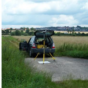
*Figure 8: Control point measurements using static GPS surveys.*
