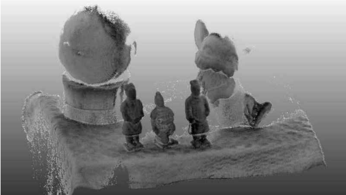
figure 3 - final point cloud determined by SCAPE from different sensor poses
