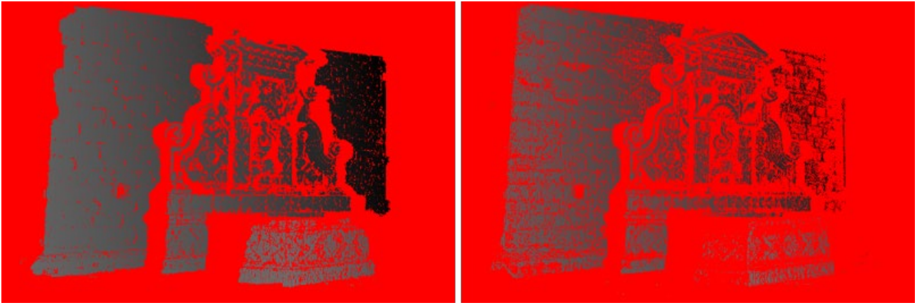
Figure 2: Depth maps generated by dense image matching. The left image shows the result of the DAISY based matching strategy. The right image is produced with a combination of Mutual Information and Census matching functions.
