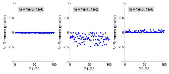
Fig. 4.5 The differences of focal length calibration vary with 100 random unknown principal points, when m is chosen as two different values.
