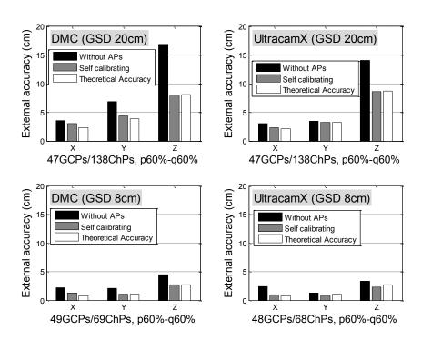
Fig. 3. 10 External accuracy in the four blocks of in-situ calibration scenarios ('without APs' indicates using the three IO parameters but not the Fourier APs).
