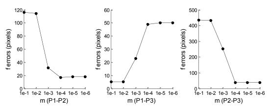
Fig. 4.4 The errors of the focal length calibration vary with different *m* in different pair views, with an unknown principal point.
