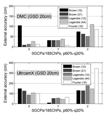
Fig. 3.16 Accuracy comparisons of different self-calibration models in the 'DMC (GSD 20cm)' (top) and 'UltraCamX (GSD 20cm)' (bottom) blocks, with zero GCP and 20% side-overlapping levels.
