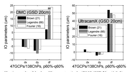
Fig. 3.17 The calibration results of the three IO parameters in the 'DMC (GSD 20cm)' (left) and 'UltraCamX (GSD 20cm)' (right) blocks of in-situ calibration scenarios.
