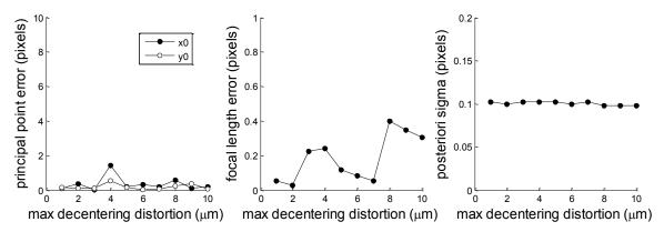
Fig. 3.24 The calibration results of principal point (left), focal length (middle) and  $\hat{\sigma}_0$  (right) vary with different decentering distortion (using the decentering distortion parameters in self-calibration).
