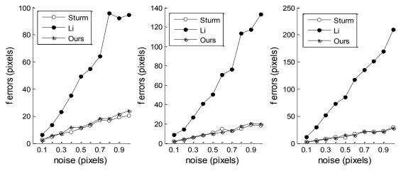
Fig. 4.3 The errors of the focal length calibration vary with different noise levels, with known principal point. The stereo views are P1\_P2 (left), P1\_P3 (middle) and P2\_P3 (right).
