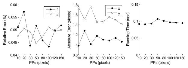
Fig. 4.11 Auto-calibration evaluation with respect to different principal point shifts.
