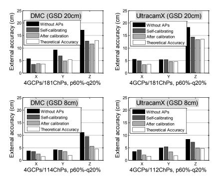
Fig. 3.9 External accuracy in the four blocks of operational project scenarios ('without APs' indicates using the three IO parameters but not the Legendre APs).
