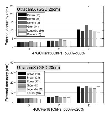
Fig. 3.15 Accuracy comparisons of different self-calibration models in the 'UltraCamX (GSD 20cm)' block of two scenarios: the in-situ calibration (top) and the operational project (bottom).
