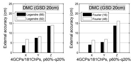
Fig. 3.21 The effects of overparameterization on the external accuracy in the DMC (GSD 20cm) block of an operational project scenario.
