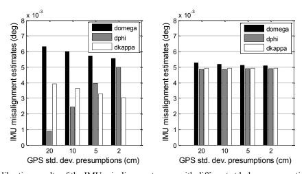
Fig. 3.5 The calibration results of the IMU misalignments vary with different std. dev. presumptions of GPS/INS position, without (left) and with (right) appropriate distortion calibration.
