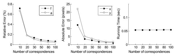
Fig. 4.10 Auto-calibration evaluation with respect to different numbers of image correspondences.
