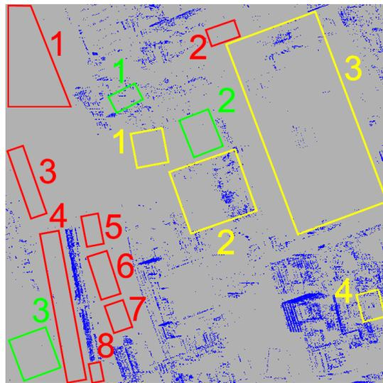
Figure 20: PS points within patch 1 (Figure 19). Building change (ground truth): red, disappearance area; green, emergence area; yellow, complex area.
