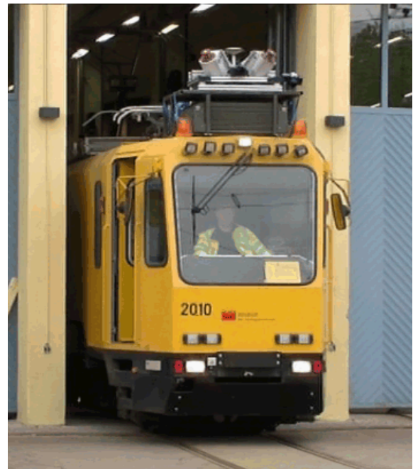
Figure 3: RailMapper as fitted to a tram in Helsinki
