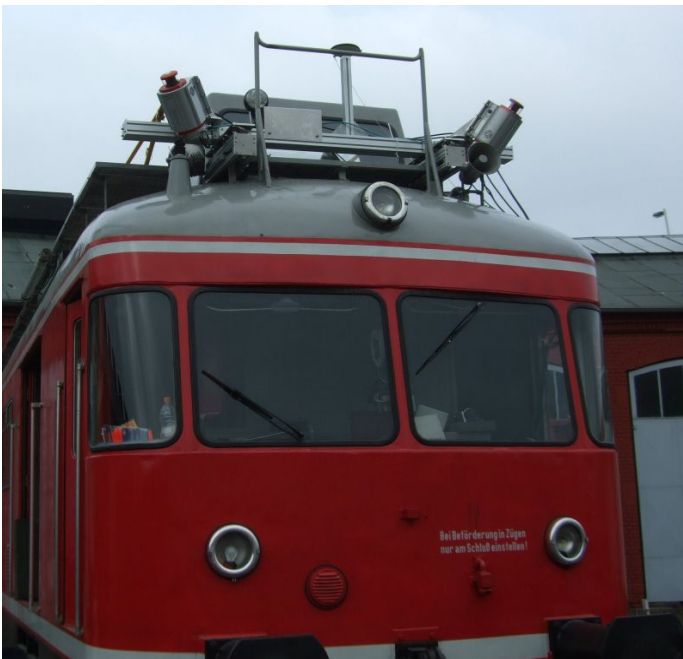
Figure 2: TVT-700 equipped with the RailMapper system
