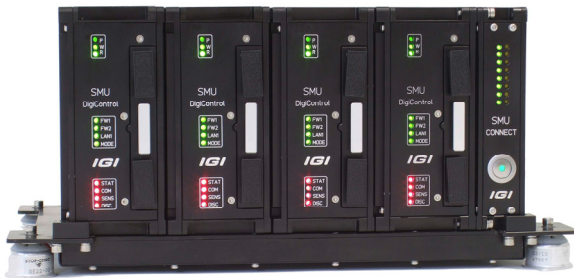
Figure 5: Quattro DigiCAM compact, rugged computer and storage unit (SMU)
