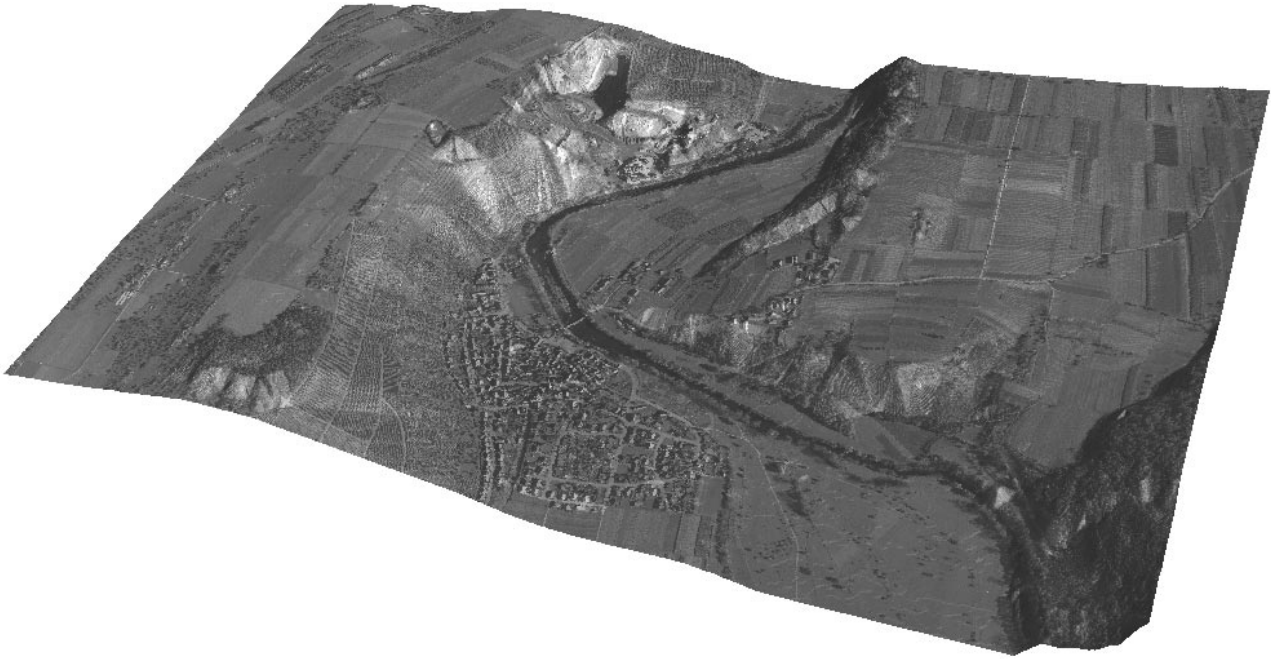
Figure 7: 3D perspective view of the ortho image draped over the DSM generated from DPA imagery
