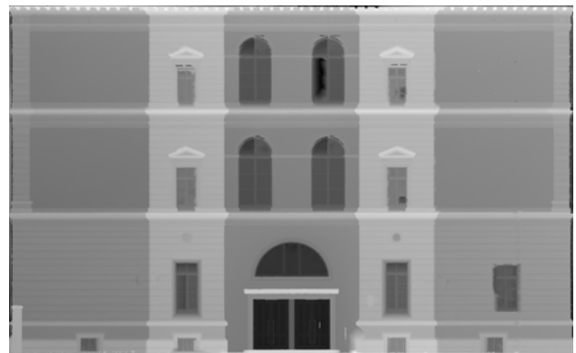
Figure 2. LASERMAP of a single facade derived from the point cloud.
