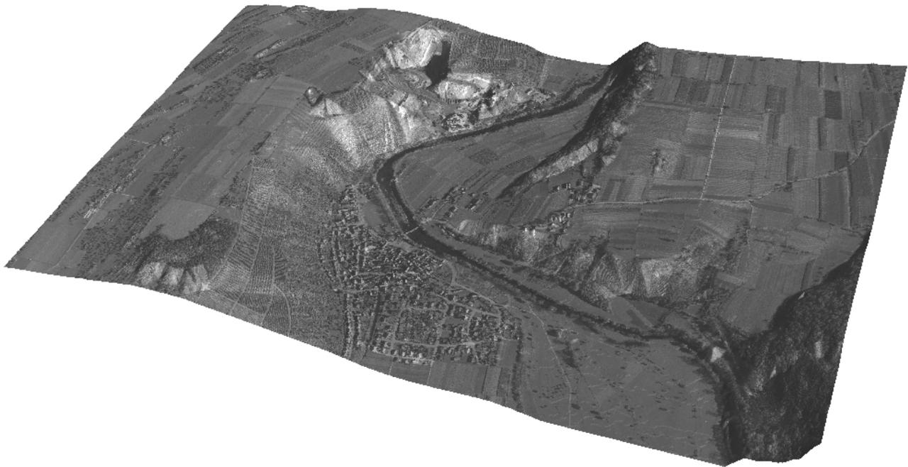
Figure 9: 3D perspective view of the ortho image draped over the DSM generated from DPA imagery
