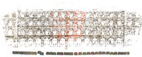
Point Cloud of a Part of Rotenhühlbau Stuttgart
