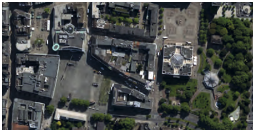
True Orthophoto with 10cm Resolution Retrieved Automatically Using SURE
