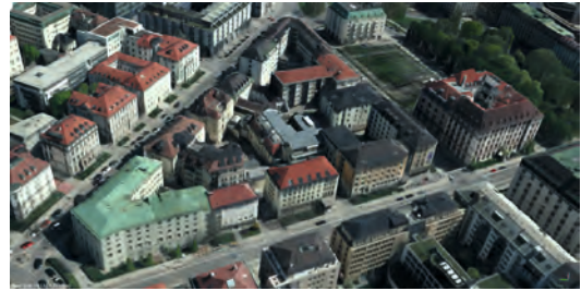
Textured Mesh of Munich, GSD 10cm, Overlap 80% in strip, 80% across strip
